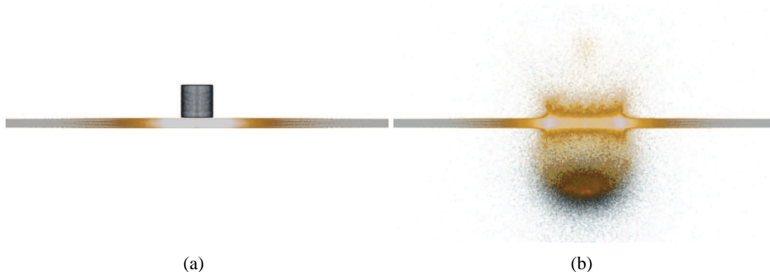
Figure 1: Snapshots of an OTM simulation of the ballistic penetration of a 152.4mm x 152.4mm x 0.5mm Al6061-T6 plate by a nylon 6/6 cylindrical projectile with length 1.8mm and diameter 1.8mm at velocity 5.2km/s. The plate and projectile are modeled by 2,042,320 material points and 1,660,470 degrees of freedom. The simulation was performed on LLNL's Hera using 2048 mpi tasks in 24 hours.
