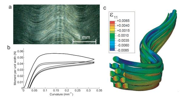
Figure 1: Folding of fiber composites with silicone rubber: (a) Micrograph of fiber microbuckling, (b) experimental moment-curvature relationship showing strain softening under cyclic loading and (c) threedimensional simulations of the folding process, with the matrix removed to aid visualization.
